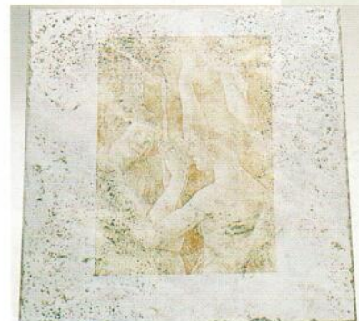
Fig. 5-35. This tile with a scanned image of a Botticelli artwork was made as a demonstration of the computer-generated decal transfer process.
