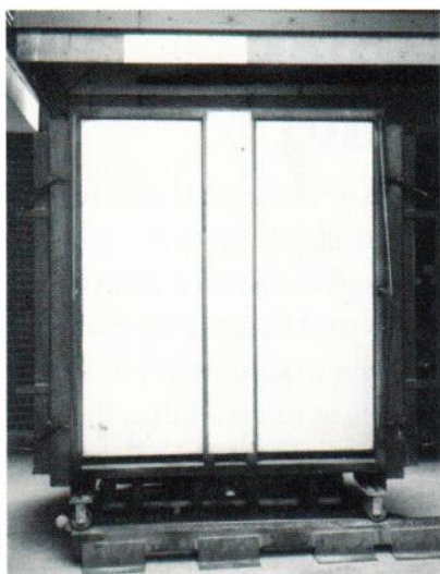
Fig. 6-5. This car kiln can accommodate a large volume of work in a short amount of time. The housing sits on a track and can be wheeled back and forth over two beds. While one bed's load is cooling, the other can be stacked.
