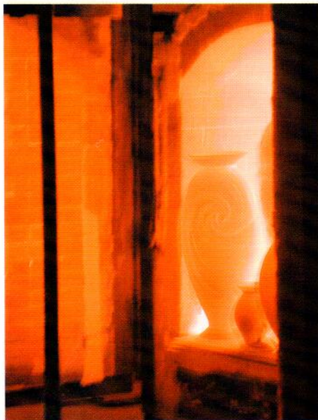
Fig. 6-41. At 1800°F, Menchhofer's large kiln is opened and the car is rolled to a post-reduction chamber. The chamber is then lowered to enclose the ware for the raku reduction process.
