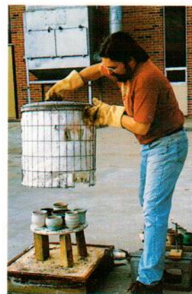
Fig. 6-52. Teacher Robert Putnam prepares a raku kiln for firing at Blue Valley High School, Stilwell, KS.
