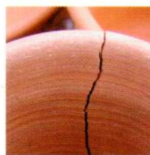
Fig. 6-40. Dunting can occur when fired clay is cooled too quickly.
