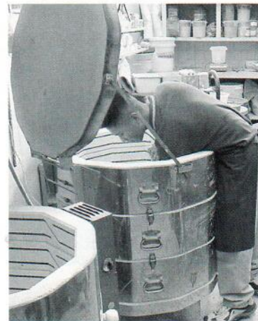
Fig. 6-4. When stacking or loading an electric kiln, leave space between the walls and the ware. Nothing should touch the electrical elements (wires) in the kiln walls. Richard Bersamina, teaching assistant. Photo by Diane Levinson.
