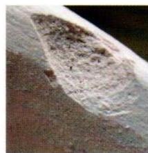
Fig. 6-39. Spalling can occur when clay is fired too fast.
