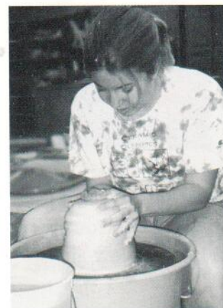
Fig. 4-7. To center more effectively, keep your hands from touching the bat or wheel head.
