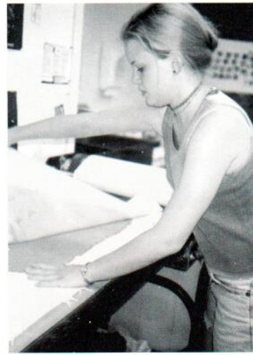
Fig. 3-30. When the clay is flattened, she reverses the direction of the wheel and rolls it back over the clay until the roller clears the slab, then removes the top canvas. The bottom canvas functions as a sling for carrying the slab to a work table.
